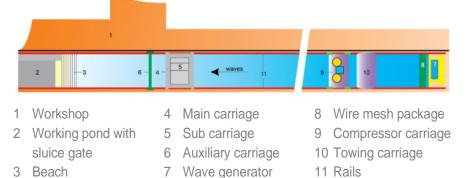
On special request MARIN might also be able to allow concept tests in the Shallow Water Basin (220 m  $\times$  15.8 m, 0-1.1 m deep).
